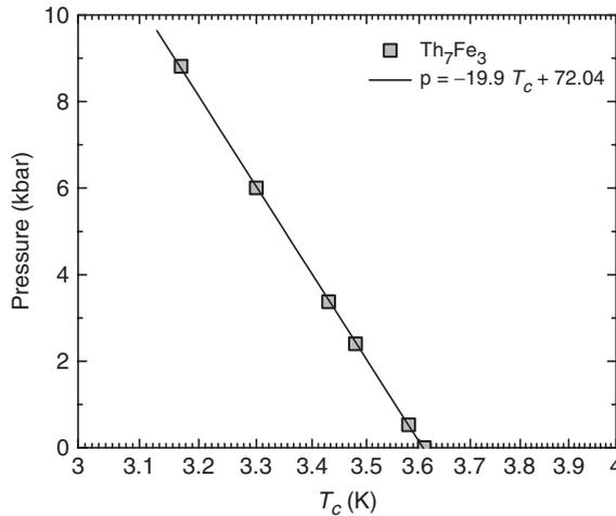
Figure 3. Pressure dependence of the superconducting transition in  $\text{Th}_7\text{Fe}_3$  up to 10 kbar. A linear fit characterizes the data over the full range of pressure.
