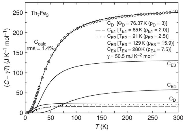
Figure 2.  $(C - \gamma T)$  vs.  $T$  for  $\text{Th}_7\text{Fe}_3$  to 300 K. Debye (for acoustic) and four Einstein (for optical) functions were used to fit the lattice data. Colour-coded curves represent the contributions of the various components with their parameters shown in the figure. The characteristic Debye temperature is  $\Theta_D$  and the Einstein temperatures are  $T_E$ .
