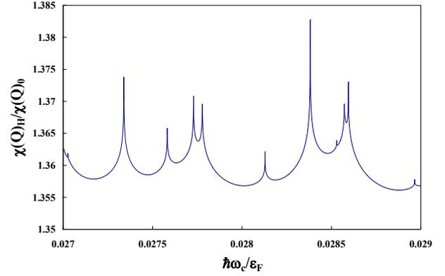
**Figure 1** The schematic field-dependence of the (normalized) density-density response function,  $\chi(\underline{Q})_H$  on  $\hbar\omega_c/\epsilon_F$ , for a general direction of  $\underline{Q}$  such as  $Q_\perp/k_F = Q_z/k_F = 1/3$ .
