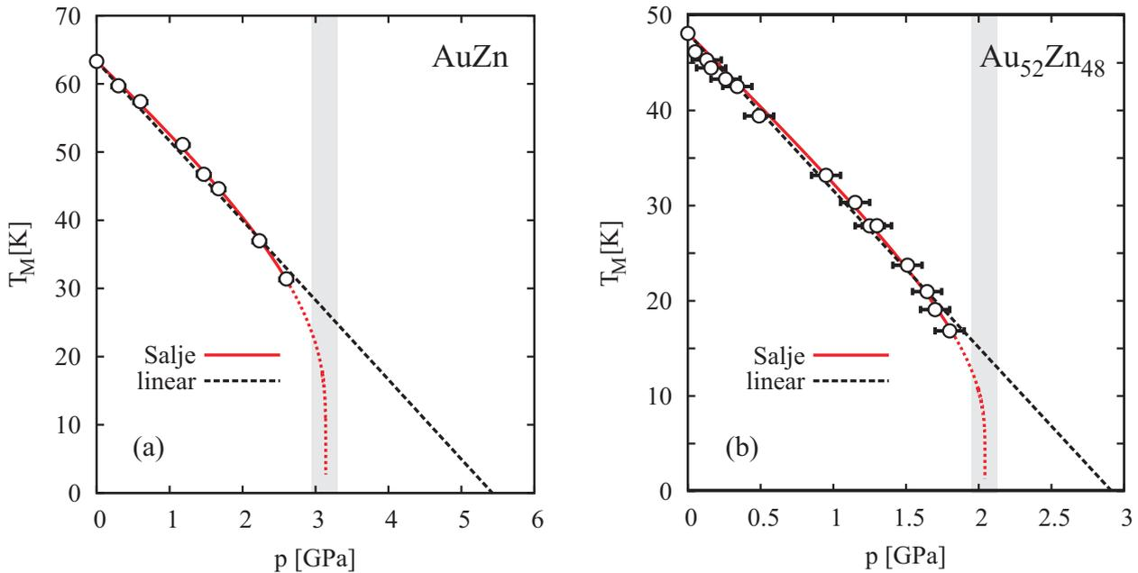
**Figure 3** The P-T phase diagram for AuZn and Au<sub>52</sub>Zn<sub>48</sub>, together with linear (black) and non-linear (red) extrapolations of the phase boundaries. The data are taken from reference [2]. The non-linear extrapolations are based on the theory of reference [12].
